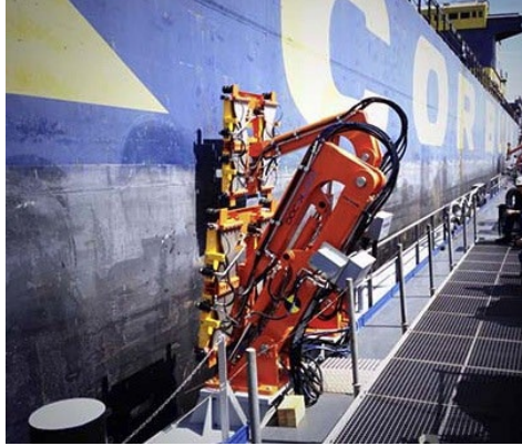
Fig.2. Electromagnetic mooring device in operation. [7]
